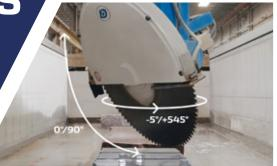
**Sliding cross-beams and bridge** with linear bearings and helicoidal-teeth racks for the X and Y axis, with lubrification by automated grease system and bellows for protection with labyrinth closure.
