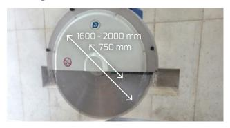
**Head up-down sliding** (Z axis) on recirculating linear ball guides with ACS safety system.
