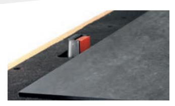
The aligning foot serves to align the sheet for the mechanical squaring of the sheet.
