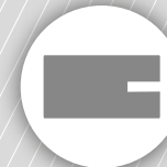
SLOT (KERF NOT PASSING RIGHT THROUGH)
