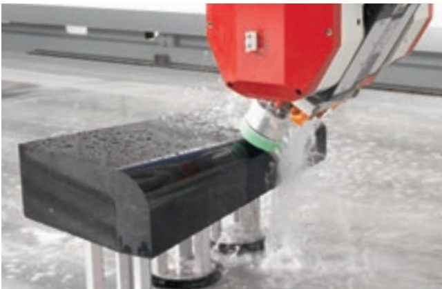
Polishing of rounded profiles on slabs.
