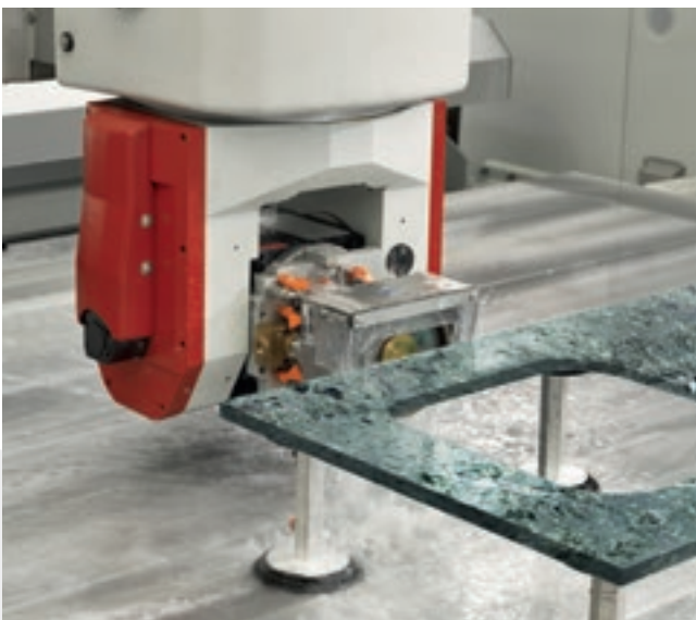
Cup grinding of the external edge.
