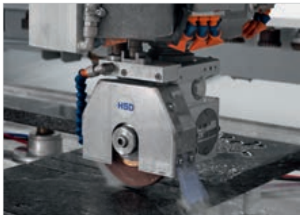
Complete external machining of kitchen tops on all sides, hole and drains polished.
