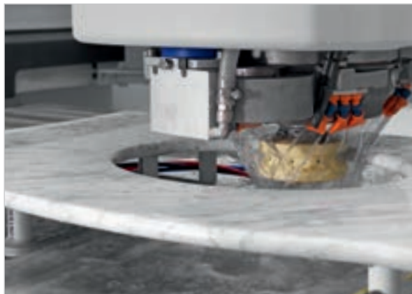
Complete external machining of kitchen tops on all sides, hole and drains polished.
