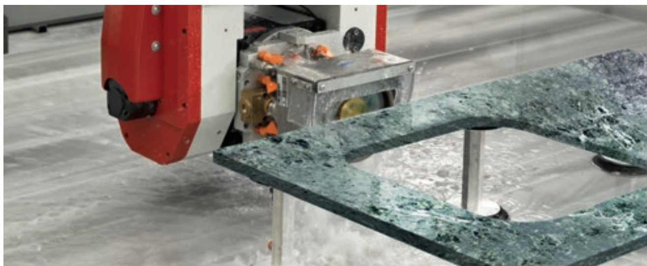
Cup grinding of the external edge.
