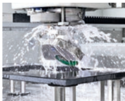
45° disc cuts for joints.
