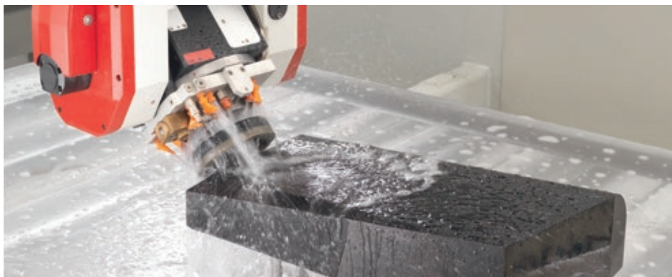
Bevel with variable angle.
