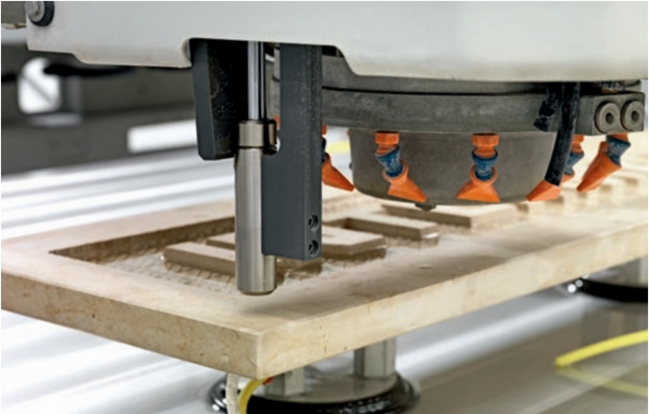
3-axis head mechanical thickness tracer.
