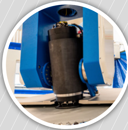
Electrospindles from 28.5 kW up to 40 kW.
