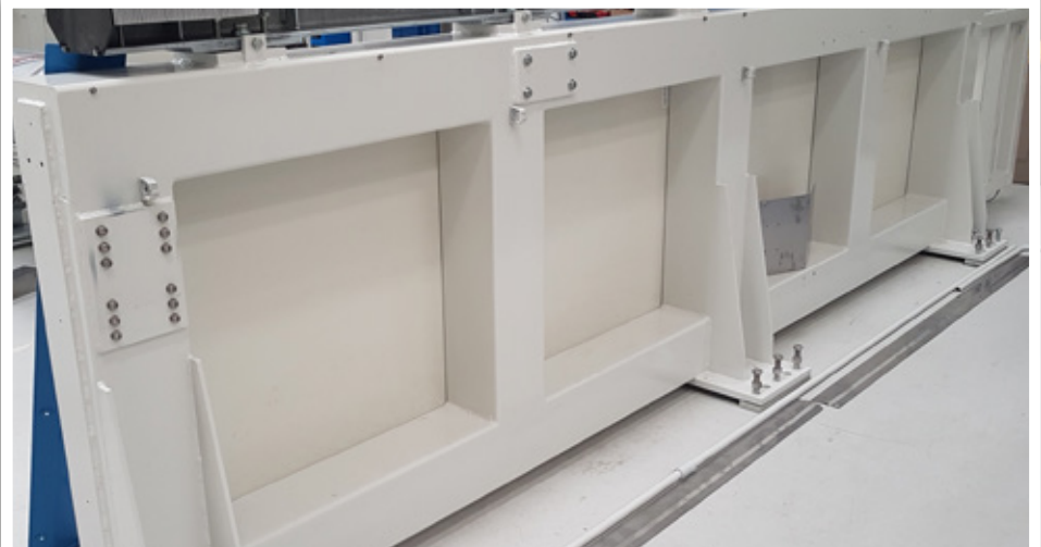
Support walls painted, normalized and sandblasted.
