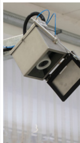
Camera for slabs: slab detection system, with camera placed above the workbench and software for image record. The application allows to speed up the machine programming.
