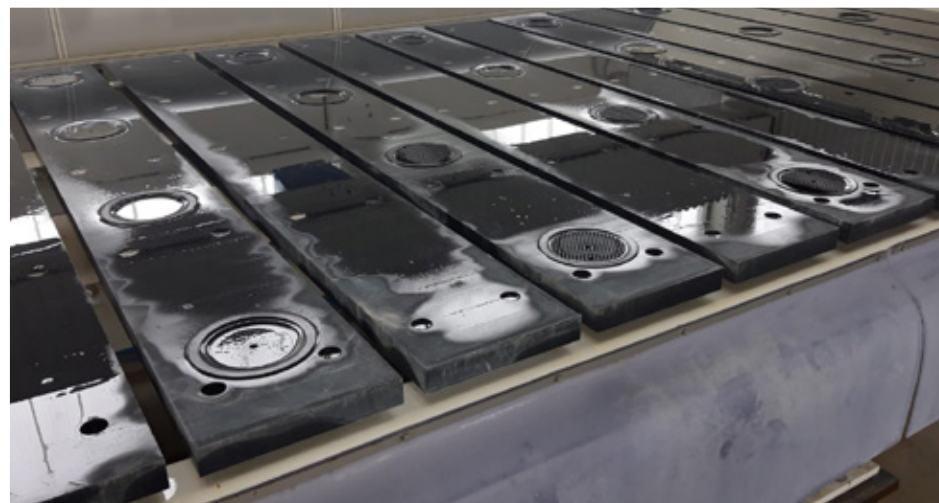
Piece fastening system with suction cups integrated on the plastic top
