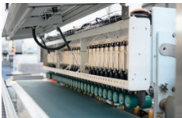
Pneumatic pressers as standard for machining panels of different thicknesses at the same time, ensuring uniform pressure which is essential when processing ceramic materials, especially those that are thin.
