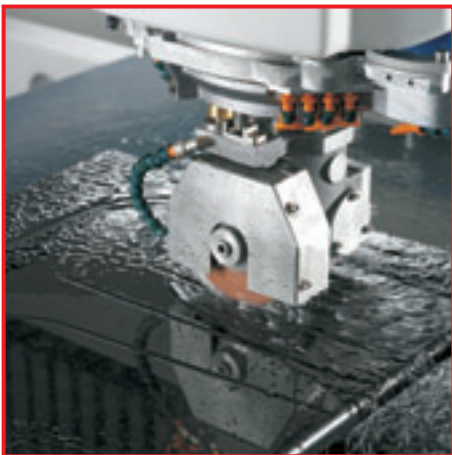
Lucidatura sgocciolatoi. Water slots polishing.
